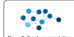
Figure D. Graph representation of thresholded functional connectivity. Edges exist between nodes (brain regions) with correlations > threshold; features are pairwise correlations.
